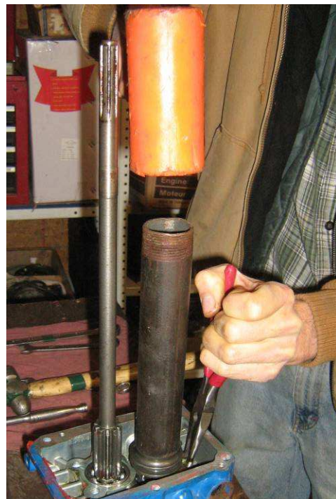
26. SET PTO SLIDER DOWN OVER PTO SHAFT (MAKE SURE IT IS RIGHT SIDE UP, AS IN PICTURE)...IT WILL REST ON TOP OF PTO TOOL "FINGERS". YOU ARE STILL COMPRESSING PTO TOOL AND HOLDING TIGHT, AND NOT MOVING, OR THE BALLS WILL POP OUT...
