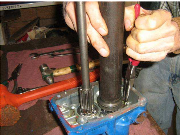
27. TAKE A PIECE OF 1 1/4" STEEL WATER PIPE (10" TO 14" LONG) AND PLACE IT ON TOP OF PTO SLIDER. NOTE DEADBLOW HAMMER TO LEFT...
