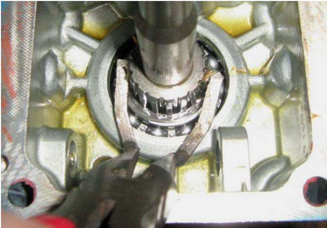
25. USING BCS "PTO TOOL" TO COMPRESS BALLS & SPRING INTO SHAFT BEFORE INSTALLING PTO SLIDER...NOTE POSITIONING OF TOOL. NOTE: IT IS BEST TO HAVE THE PTO SHAFT END THAT IS PROTRUDING THROUGH THE COVER CLAMPED IN A VISE FOR THIS PROCEDURE, TO HOLD IT AND THE COVER STILL...THIS PIC WOULD BE LOOKING DOWN.
