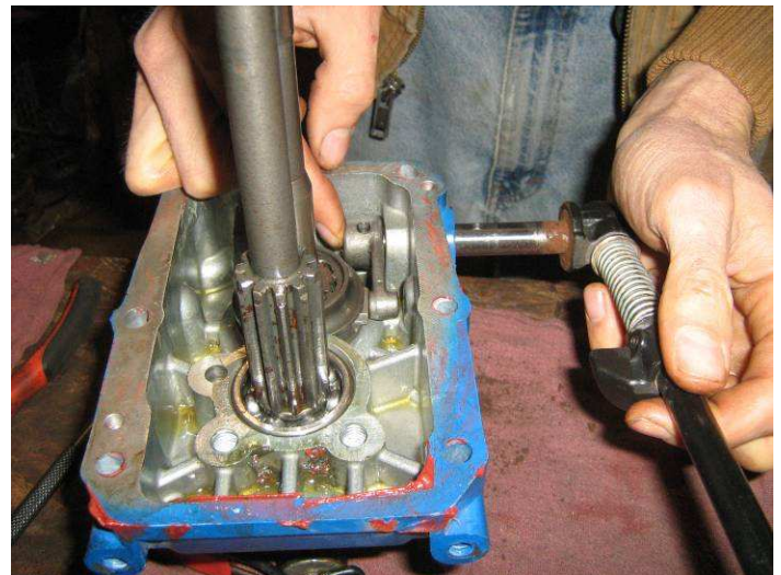
32. INSERT OUTER PTO LEVER THROUGH HOLE IN HOUSING, ALIGNING WITH INTERNAL LEVER ( NOTE: IF YOU HAVE REPLACED THE PTO COVER, MAKE SURE YOU HAVE INSTALLED THE LITTLE OIL SEAL IN THE HOLE WHERE THIS LEVER COMES THROUGH THE HOUSING, OR YOU WILL HAVE AN OIL LEAK!!)
