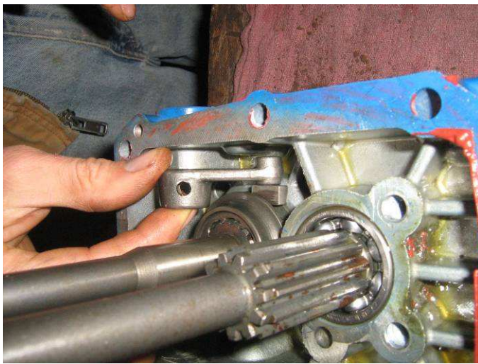
31. SET INTERNAL PTO LEVER DOWN INTO HOUSING, ENGAGING SHOE INTO GROOVE IN SLIDER
