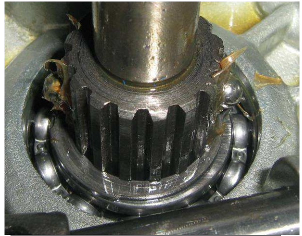
24. BALLS STUCK IN GREASE ON EITHER SIDE OF HOLES IN SHAFT; SPRING IS INSIDE SHAFT (BETWEEN BALLS)
