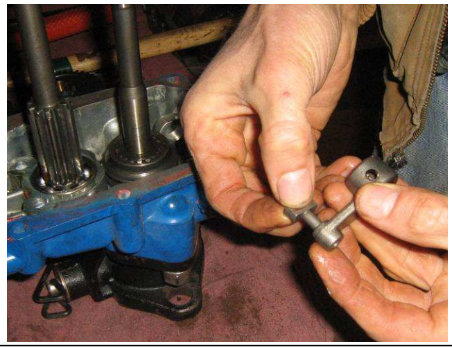
30. INSERT "SHOE" INTO INTERNAL PTO SHIFT LEVER...MAKE SURE TO GET IT IN CORRECT SIDE!!
