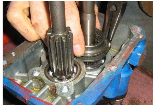
26. SET PTO SLIDER DOWN OVER PTO SHAFT (MAKE SURE IT IS RIGHT SIDE UP, AS IN PICTURE)...IT WILL REST ON TOP OF PTO TOOL "FINGERS". YOU ARE STILL COMPRESSING PTO TOOL AND HOLDING TIGHT, AND NOT MOVING, OR THE BALLS WILL POP OUT...
