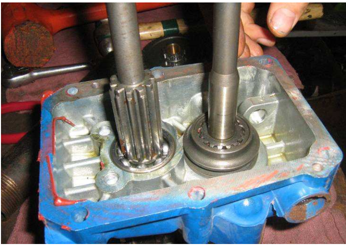
29. PROPERLY INSTALLED PTO SLIDER (AFTER PTO TOOL MANEUVERED OUT FROM UNDER IT)
