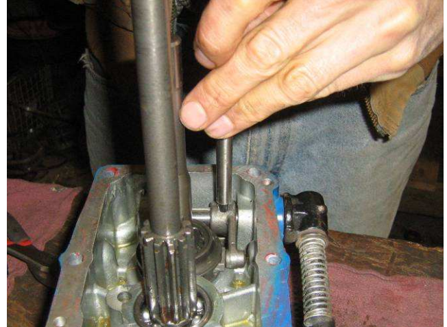
34. ...AND DRIVE DOWN FLUSH WITH PIN PUNCH AND (STEEL) HAMMER. MAKE SURE YOU DON'T ACCIDENTALLY "SHIFT" THE PTO LEVER WHILE THE COVER IS STILL OFF THE TRACTOR...YOU MIGHT POP THE PTO SLIDER OFF THE BALLS, AND HAVE TO DO THAT ALL OVER AGAIN!!
