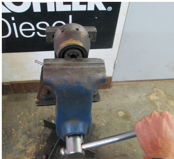
Tighten the vise...you may have to really crank down on it to get the clutch to break loose. You can generate many more times the force with the vise than you can with the clutch linkage on the tractor. When it breaks free, you will undoubtedly hear a load “POP” or “BANG”...don't freak out!
