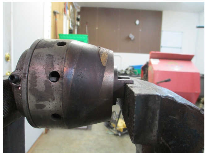
Side view of clutch in vise. One of the vise jaws is against the hole where the clutch came off the engine, and the other vise jaw is against the flat pad on the throwout-bearing plate. NOTE: we are NOT pushing on the two little “tabs”—they are rotated so they are up over the vise jaw.
