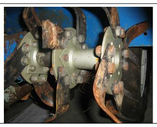
**INDIVIDUAL:** Tines bolt on individually, not sharing any mounting bolts. 8 bolts per full set of 4 tines.
