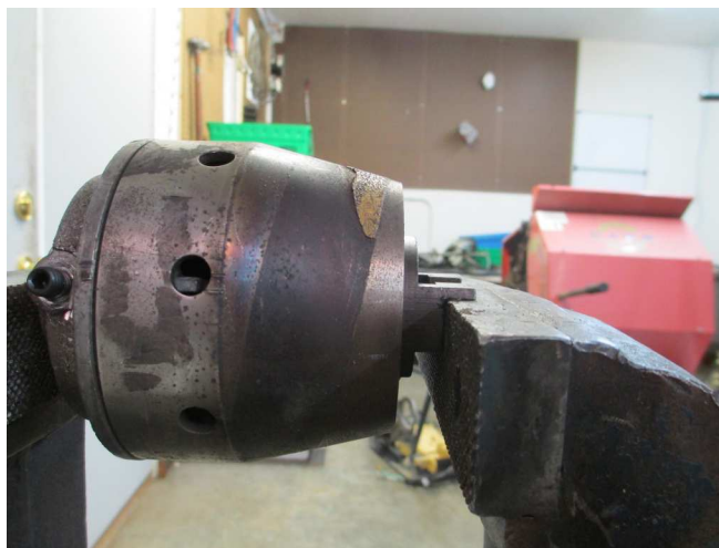
Side view of clutch in vise. One of the vise jaws is against the hole where the clutch came off the engine, and the other vise jaw is against the flat pad on the throwout-bearing plate. NOTE: we are NOT pushing on the two little “tabs”—they are rotated so they are up over the vise jaw.
