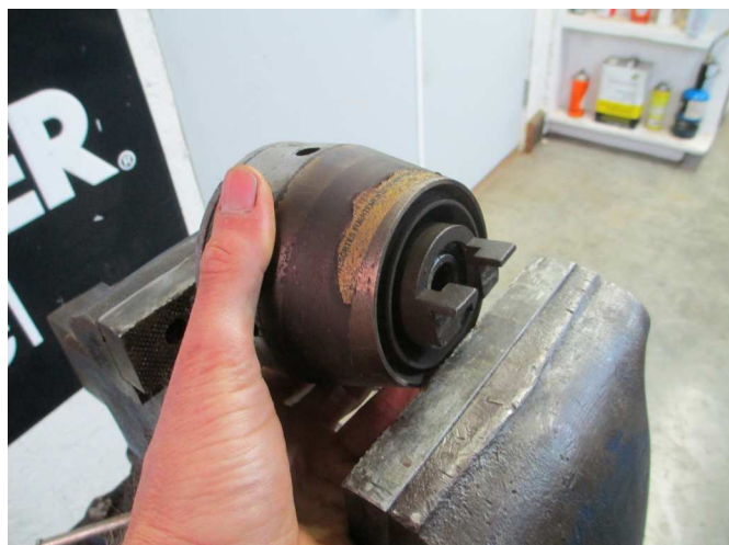
After removing the stuck clutch from the engine, place the clutch in a vise, front-to-back.
