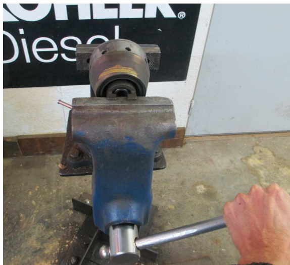
Tighten the vise...you may have to really crank down on it to get the clutch to break loose. You can generate many more times the force with the vise than you can with the clutch linkage on the tractor. When it breaks free, you will undoubtedly hear a loud “POP” or “BANG” ...don't freak out!
